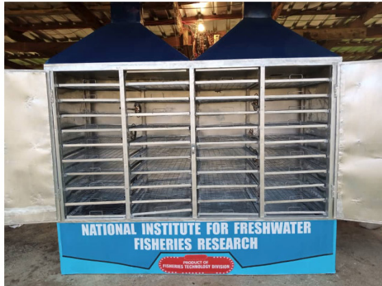
Inside view of 500-750kg Electric/Gas/Charcoal Energy Sources HYBRID FISH SMOKING KILN OF NIFFR-WAAPP
