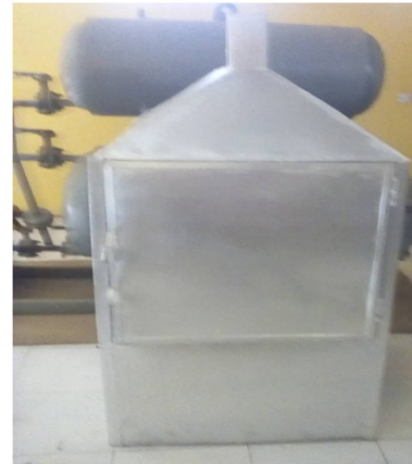
Front view of 250-350 kg Electric/Gas/Charcoal Energy Sources HYBRID FISH SMOKING KILN USING GAS
